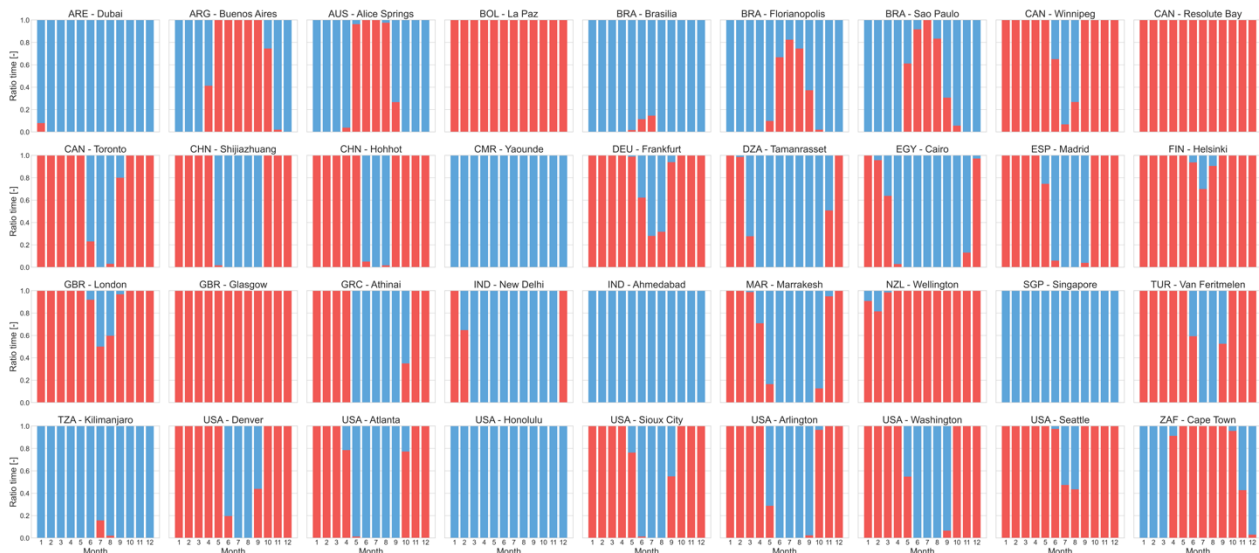
Figure 1: Flexible definition of heating and cooling seasons across samples in all ASHRAE 169-2021 climate zones: proportion of HDD and CDD per month (red: HDD relative influence, blue: CDD ones)
